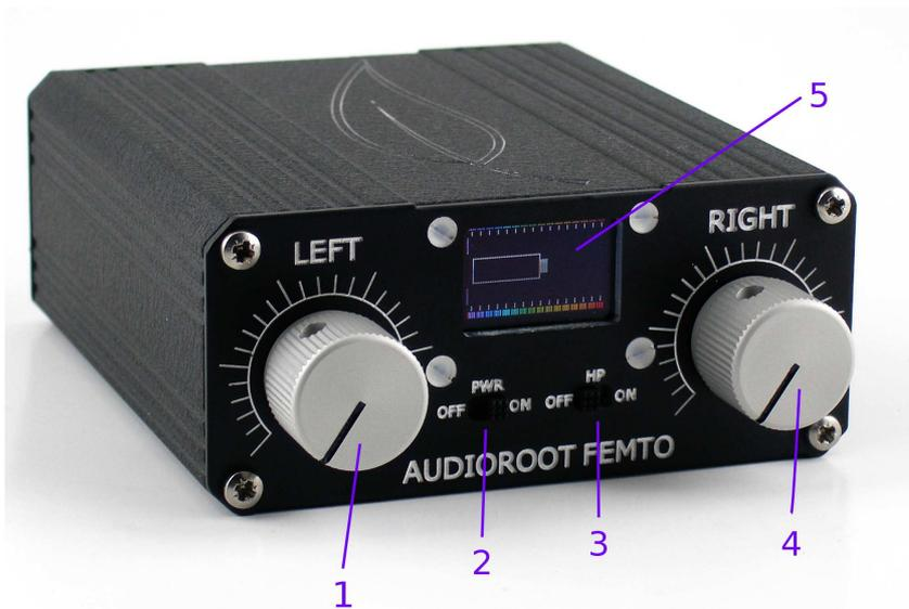
1. **Left** input gain level adjustment potentiometer. Gain can be adjusted from +10dB to +64dB. Please note that left and right channel gains cannot be stereo linked (ganged) on the Femto
