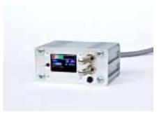
minutes. A nice bright red LED will flash when you get below ten percent capacity. There is a regulated version available with two 9v outputs for directly powering radio mic receivers.
